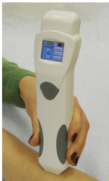
Figure 4 Skintel pigment meter in action—the device reports a value between 10 and 100.
